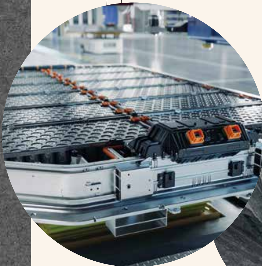
Lithium-ion high voltage battery for electric vehicle.
